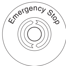
Figure 19. Emergency Stop Switch
