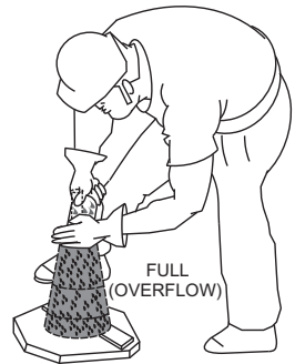
Figure 68-C. Slump Test (Full-Overflow)
