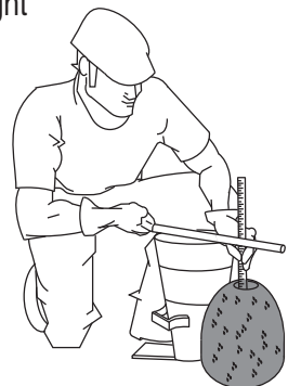
Figure 68-F. Slump Test (Measurement)
