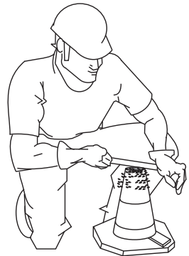
Figure 68-D. Slump Test (Removing Excess Concrete)
