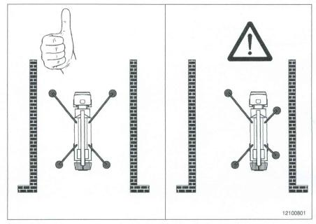
The support legs must always be fully swung out and extended
