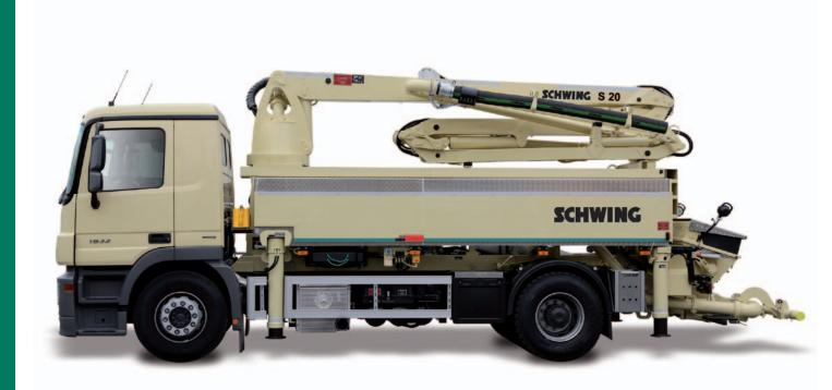
Permanently mounted hose boxes ensure convenient access to 100 m of hose up to DN 75 on the left side and 36 m of hose up to DN 100 on the right side.
